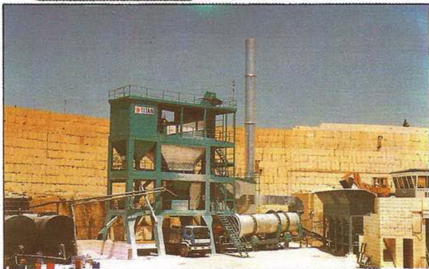
TITAN 2000 Hot Asphalt Mixing Plant - The only one of its kind in Malta.
